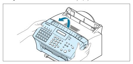
2. Remove the old toner cartridge. Follow the instructions printed on the cartridge box to recycle the used cartridge.
